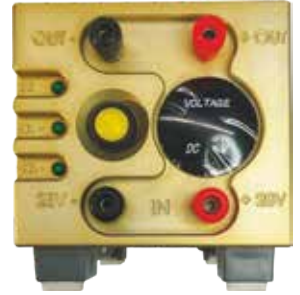
TÜRK HAVA YOLLARI COCKPIT KAPI KİLİT TEST CİHAZI
